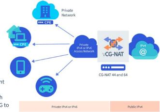
6WIND vCG-NAT works as a Virtual Machine on top of standard x86 server to provide flexibility and cost-efficiency for small and large deployments.
